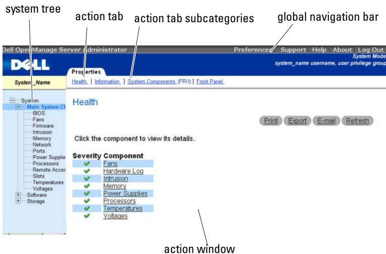
Figure 4-1. Sample Server Administrator Home Page — Non-Modular System
